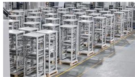
Masterlan free-standing outdoor cabinet 19" 42U/800mm, assembled.
